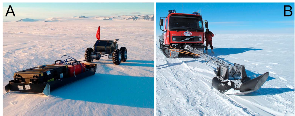
Figure 19. (a) An autonomous ground-penetrating radar unit (Yeti) being used to map near-surface buried crevasses at White Island, Antarctica, in October 2014. (Photo: Jim Lever) (b) High-frequency ground-penetrating radar pushed by a vehicle on the Norway-USA Scientific Traverse of East Antarctica during the International Polar Year, in November 2008. (Photo: Ted Scambos).
