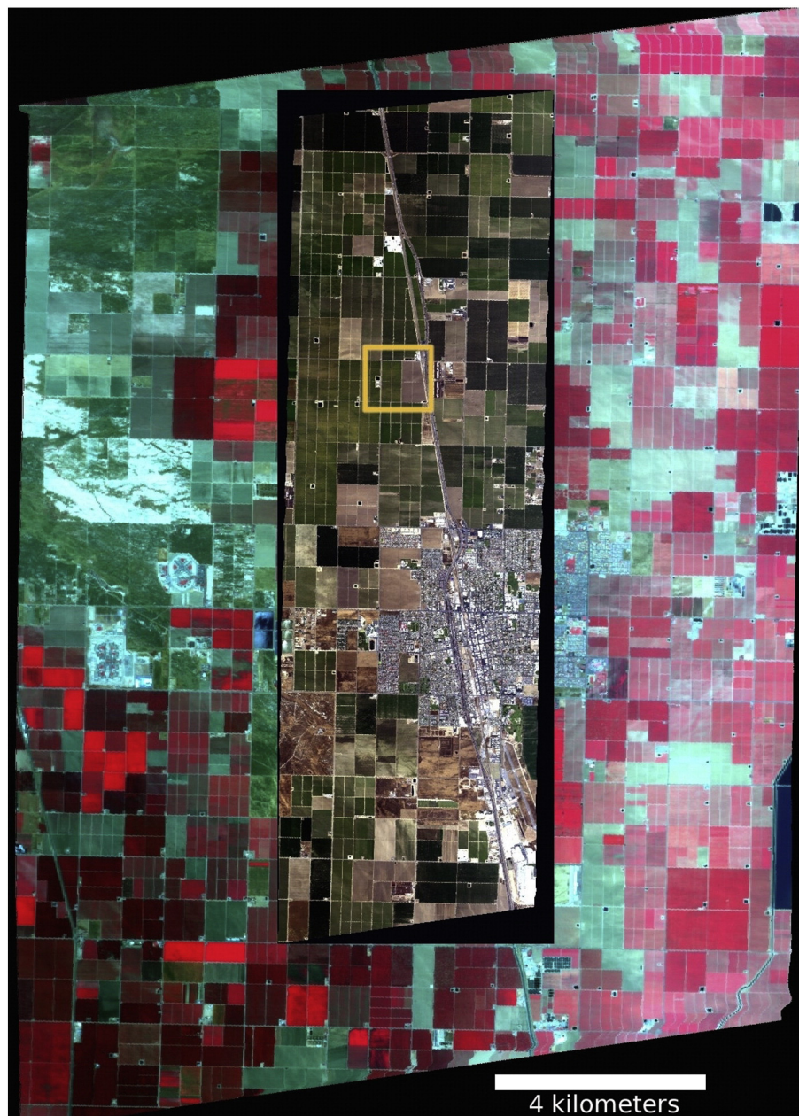
Fig. 2. MASTER and AVIRIS flight lines; yellow box is the field site shown in Fig. 1. MASTER bands: Red = 9, green = 5, blue = 3; AVIRIS bands: red = 29, green = 20, blue = 11.
